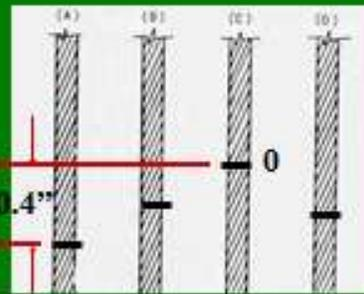
Using the parameters shown in our scenario, the maximum allowable mark displacement during the test is 0.322" and in order to correct this mark displacement, we would in theory have to cut the groove by 0.023". Normally, it is good practice to cut the long groove (the lowest shown) by half of the theoretical value and perform another test.
